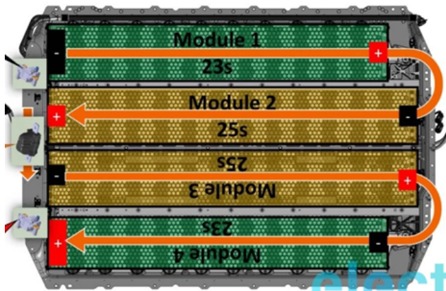
Figure 2. Battery layout in the Tesla Model 3 long range[1].
